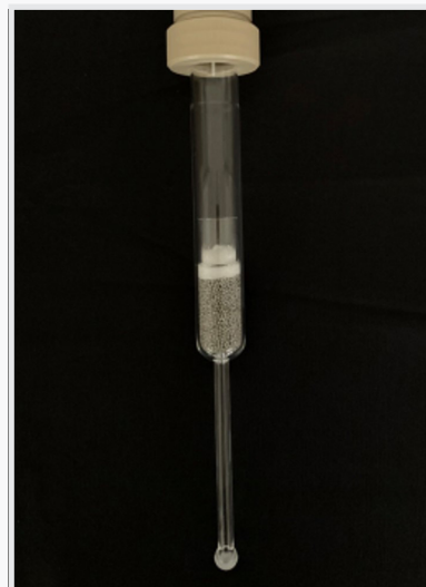
Figure 2: Image of the salt combustion tube, part of the salt kit.
