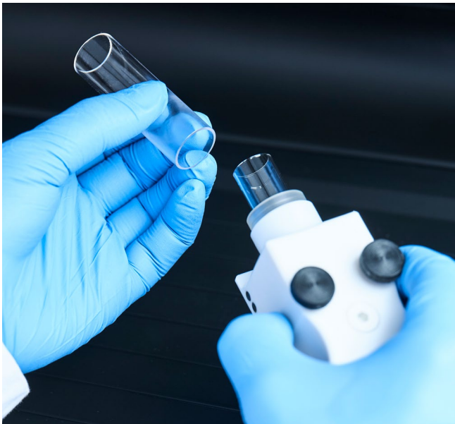
Modular demountable torch (V Shuttle Torch)
