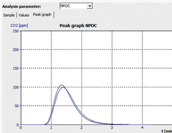
Figure 3: Measurement curves "matrix + 1000 ppb KHP"
