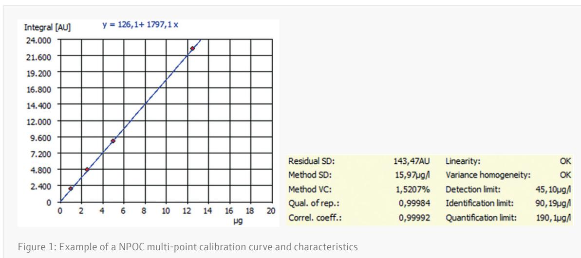
Figure 1: Example of a NPOC multi-point calibration curve and characteristics
