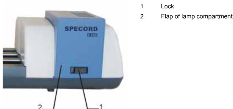
Fig. 12 Opening the flap of the lamp compartment
