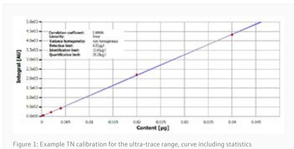
Figure 1: Example TN calibration for the ultra-trace range, curve including statistics
